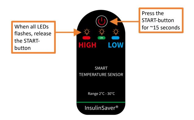
To turn off your InsulinSaver, press and hold the START button for approx. 15 seconds. When all the LEDs are flashing, release the START button.
